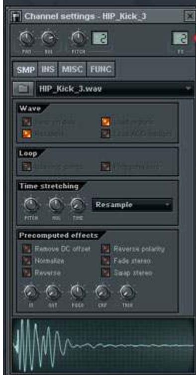
FX number sends channel to specific mixer insert, where FX can be added. Here FX 2 to Insert 2
